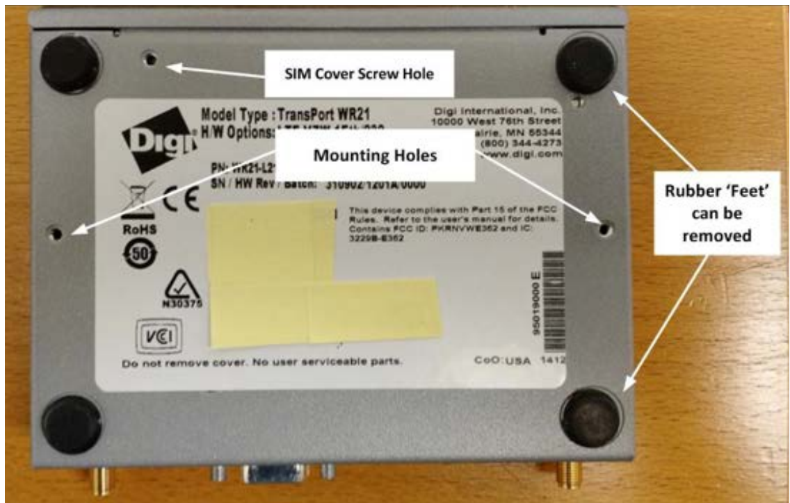
Bottom view of a Digi TransPort WR21.
