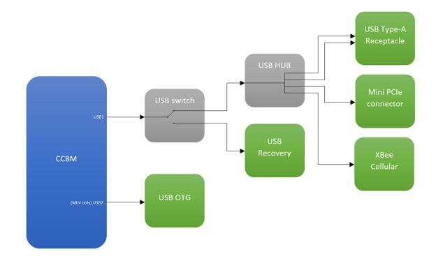
**Note** If J36 is closed, then the USB1 bus of the CPU is forced to be connected to the recovery connector J35.
