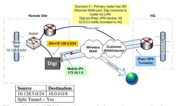
Why use this method? This is somewhat a comprise between the two approaches above. It still allows split tunneling but simplifies the VPN policy configuration and helps facilitate a "flat" network.
