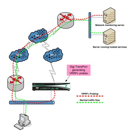
The diagram above shows the path of the VRRP+ probes sent from the Digi TransPort to a host on the remote network and the path of normal data traffic.
