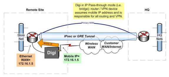
Here the primary router/VPN device controls all traffic except for management traffic to the Digi device itself via management *pinholes*.
