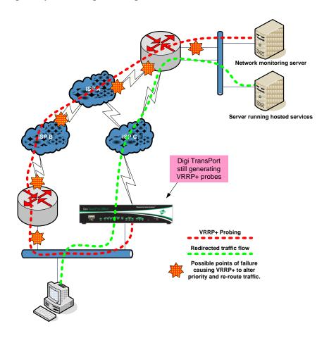
The above diagram shows the TransPort assuming the master router role while continuing to send probes.
